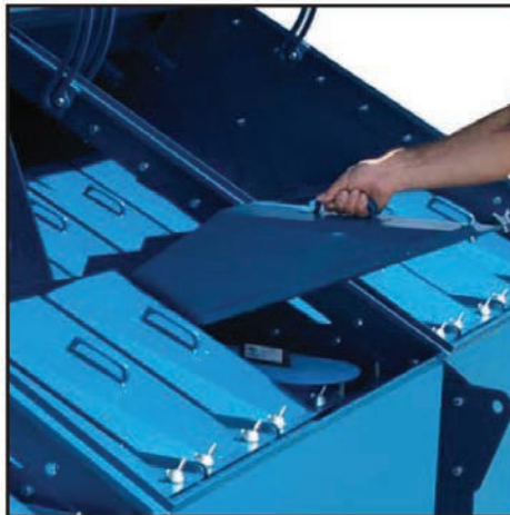
Loosen the captive hardware and remove the filter retainer/accumulator.
